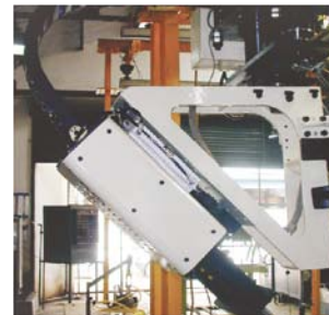
3 Spindle DC Nutrunner for Spark Plug Tightening
