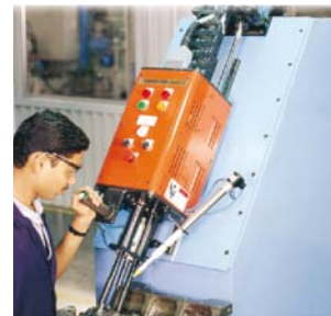
2 Spindle DC Nutrunner for Connecting Rod Tightening
