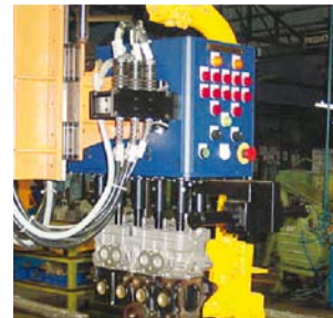
12 Spindle DC Nutrunner for Cylinder Head Tightening
