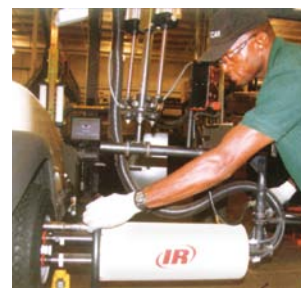
4 Spindle for Wheel Nut Tightening
