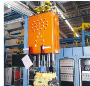
18 Spindle DC Nutrunner for Cylinder Head Tightening
