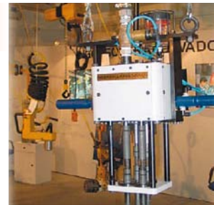
4 Spindle air Nutrunner for Cylinder Head Tightening
